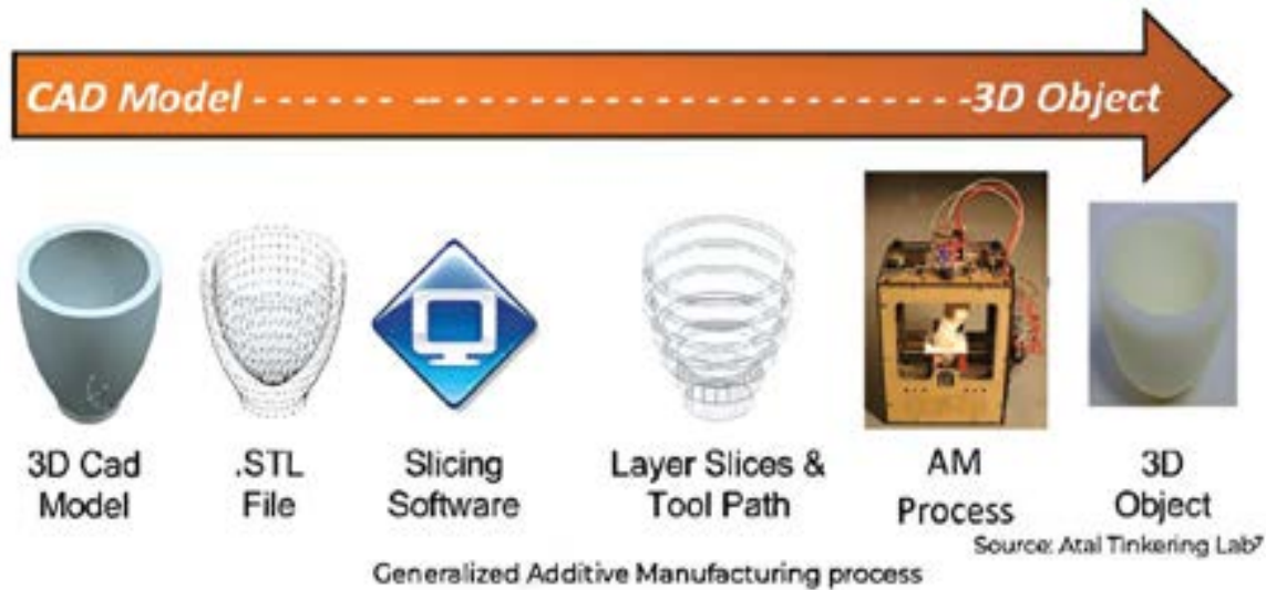
Fig.6 Basic Additive Manufacturing process
